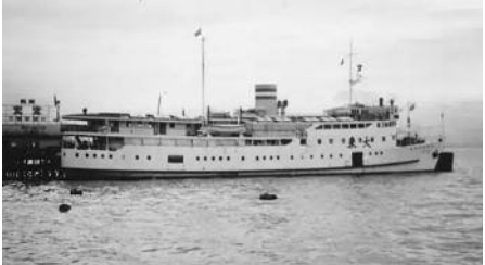
The Tai Loy, built in Hong Kong by Wing On Shung Shipyard. She was laid down in 1948, launched in 1949 and went into full service in 1951. She was a modern, purpose built triple screw motor ship of the times. In imperial measurements she had an overall length of 200ft and beam of 36ft GRT 1,330. The vessel was later renamed Nam Shan and became famous for her appearance in the 1975 French Movie "Emmanuelle 2", which was filmed in Hong Kong.
