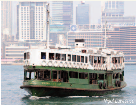
A modern day ferry. Note the navigating bridge fore and aft on the lower deck. Upper deck was for First Class and Lower deck Second Class. True icons of the World's most photographed port. There are currently 9 diesel-electric Ferries in the Star Ferry fleet, with the same basic design features remaining. The numbering followed by the letter "P" painted on the hull, denotes the number of passengers the ferry is certified to carry.
