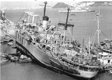
A dramatic image above of the 7,606grt USS Regulus (ex Escanaba Victory) firmly aground on 17th August during Typhoon Rose, at Kau I Chau Island. The grounding caused massive hull damage to the ship and after 3 weeks attempting to salvage her it became obvious it was unviable and she was declared a total loss, subsequently being struck from the USN list. The vessel was progressively demolished in situ.
