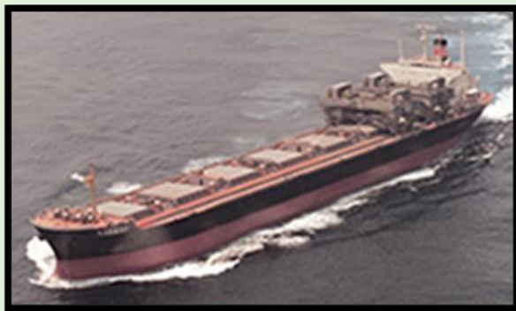
See left, 1970 heralded the delivery of Iino Line's Zenkoran Maru NO. 5 (58,931 dwt), the Group's first Panamax dry bulk carrier. This vessel was fitted with gantry cranes, allowing self – discharge.
